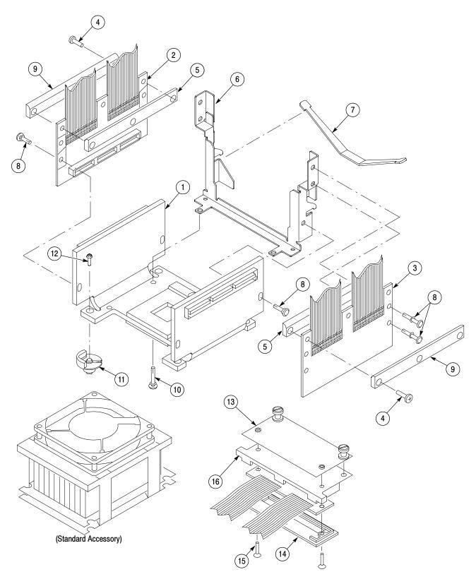
Figure 5-1: 478 Pin Socket probe adapter exploded view
