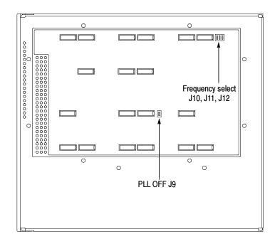
Figure 1-2: Jumper locations on the preprocessor unit
