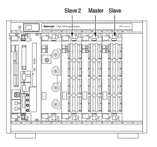
Figure 1-3: Configuration for master and slave modules
