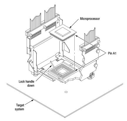
Figure 1-7: Connecting the microprocessor, probe head, and target system
