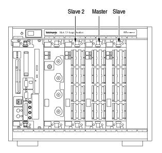
Figure 3-1: Configuration of the master, slave, and slave 2, modules
