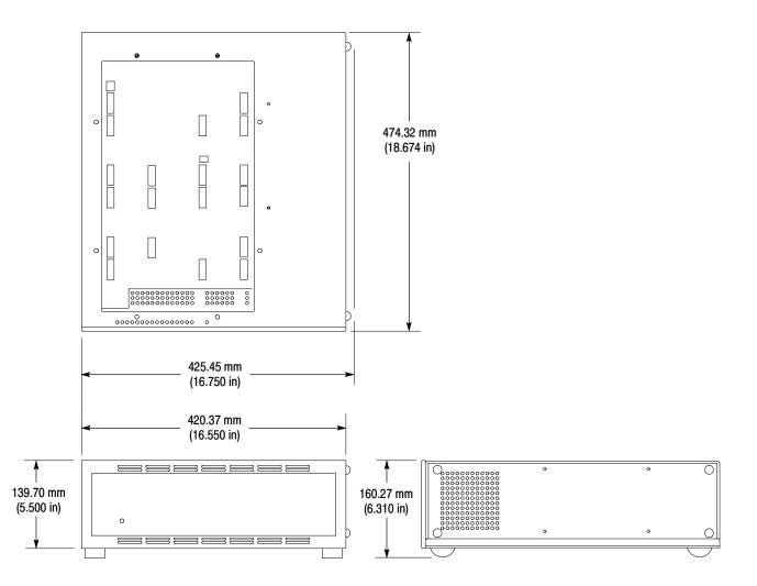
Figure 2-7: Dimensions of the preprocessor unit
