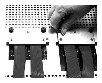
Figure 4-12: Attach the cables to the logic board cover plate
