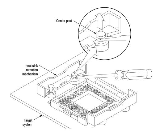
Figure 1-4: Removing the heat sink retention mechanism from the target system
