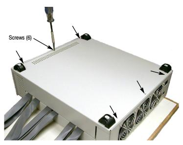
Figure 4-16: Remove the attaching screws
