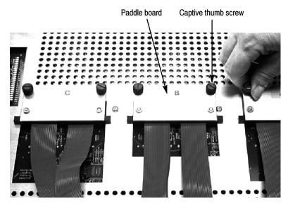
Figure 4-5: Remove the cables from the logic board
