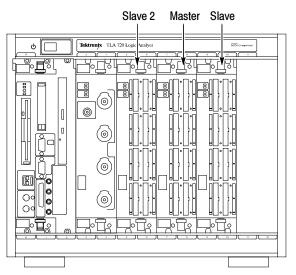
Figure 1-11: Configuration of the master, slave, and slave 2 modules
