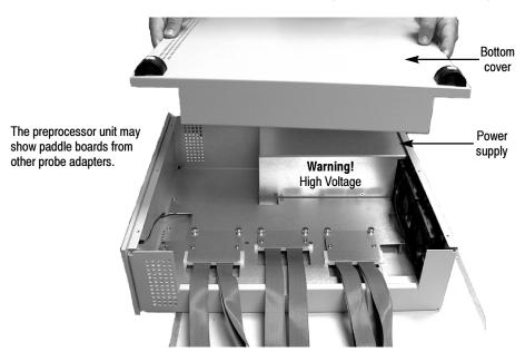
Figure 4-4: Remove the bottom cover
