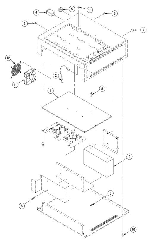
Figure 5-2: Preprocessor unit exploded view
