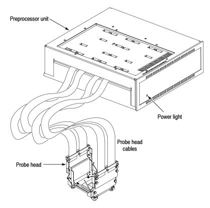
Figure 4-1: Probe head and preprocessor unit
