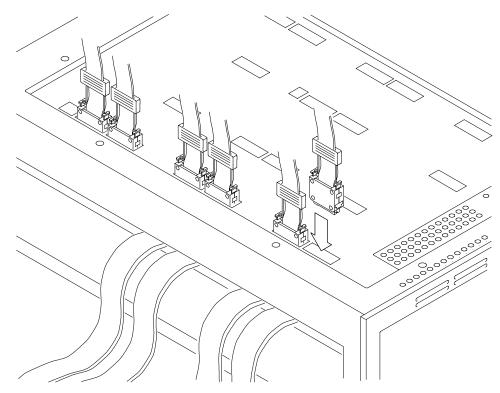
Figure 1-10: Connecting probes
