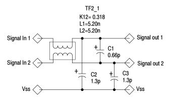
Figure 2-3: ZIF electrical load model for typical signals
