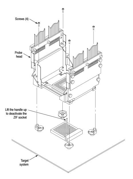
Figure 1-6: Connect the probe head to the target system
