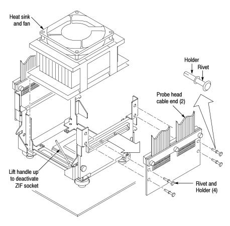
Figure 4-6: Remove the cables from the probe head
