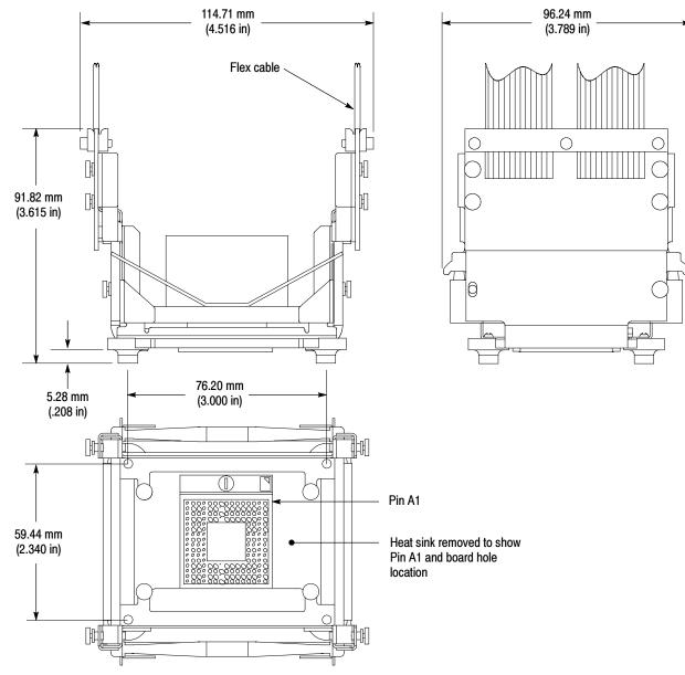
**Dimensions** Figure 2-6 shows the dimensions of the 478 Pin Socket probe head.
