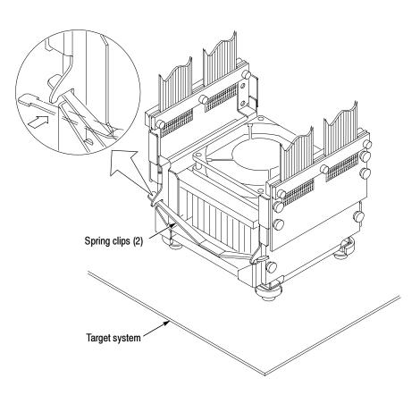
Figure 1-9: Attaching the spring clips to the heat sink
