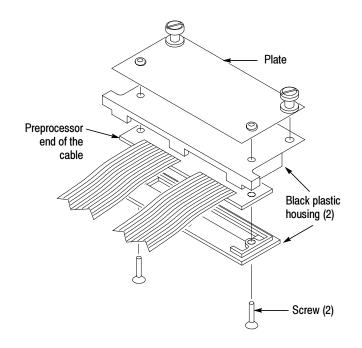
Figure 4-8: Preprocessor cable end
