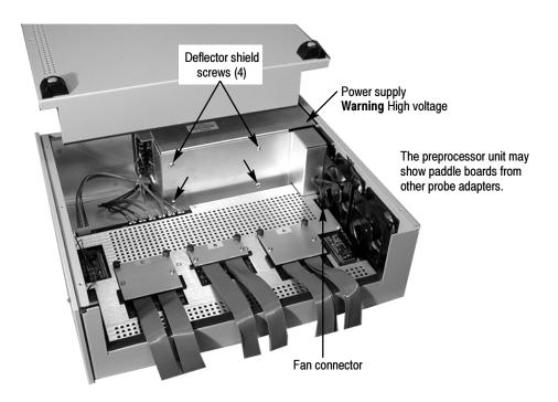
Figure 4-17: Remove the bottom cover
