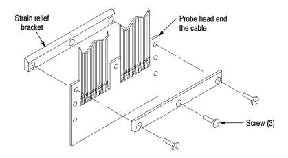
Figure 4-7: Probe-head cable end
