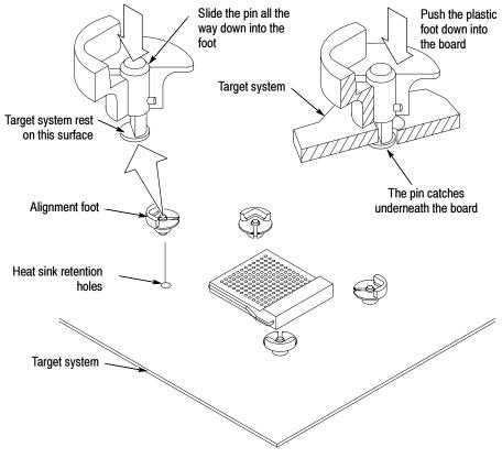
Figure 1-5: Install the base-bracket feet
