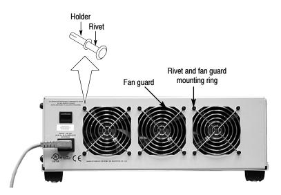
Figure 4-19: Back of the preprocessor unit
