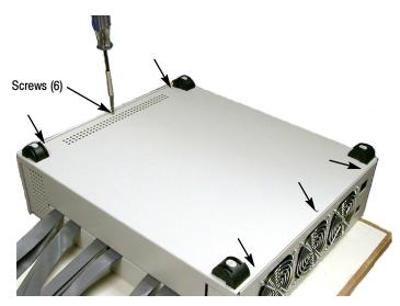
Figure 4-3: Remove the attaching screws
