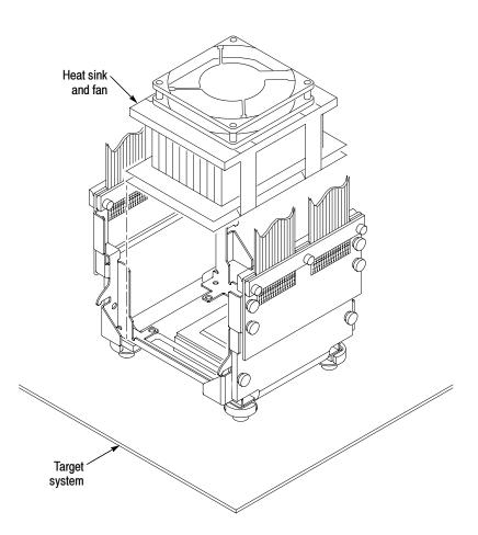
Figure 1-8: Placing the heat sink on the probe head
